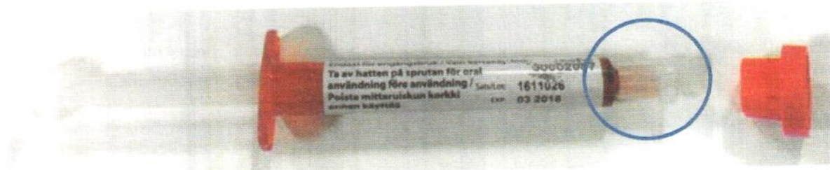
Figure 2. Upon removing the red cap, the translucent tip-cap remains on the syringe (abnormal removal reported) for illustrative purposes, not UK pack
